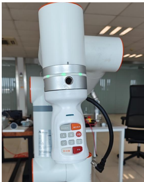
Figure 1.6 Installed Smart Tool Component
