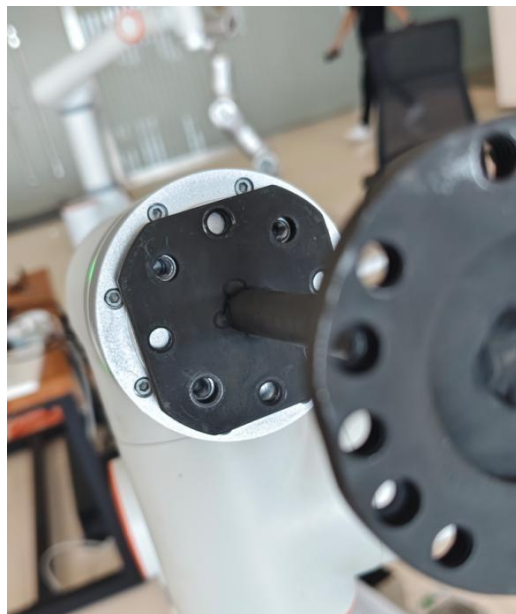
Figure 1.5 Screw Hole Alignment Between Robot End and TCP Connector
